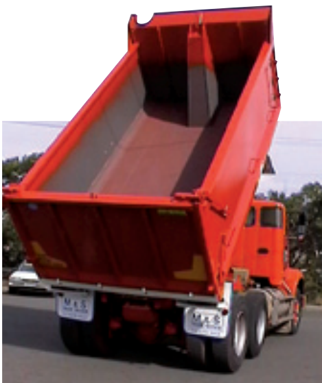
Bisplate's strength and hardness gives far greater resistance to denting than mild steel – in turn resulting in less "hang up" when carrying "sticky" loads.
