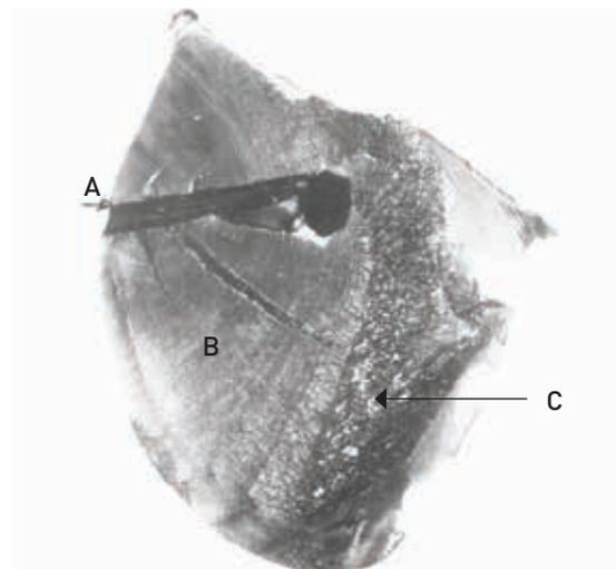
Fatigue fracture surface of a failed gear showing the concoidal “beach markings” radiating from the oil hole, marked (A). Also shown are the “beach markings” associated with fatigue crack growth (B), and the area where ductile overload occurred (C).
