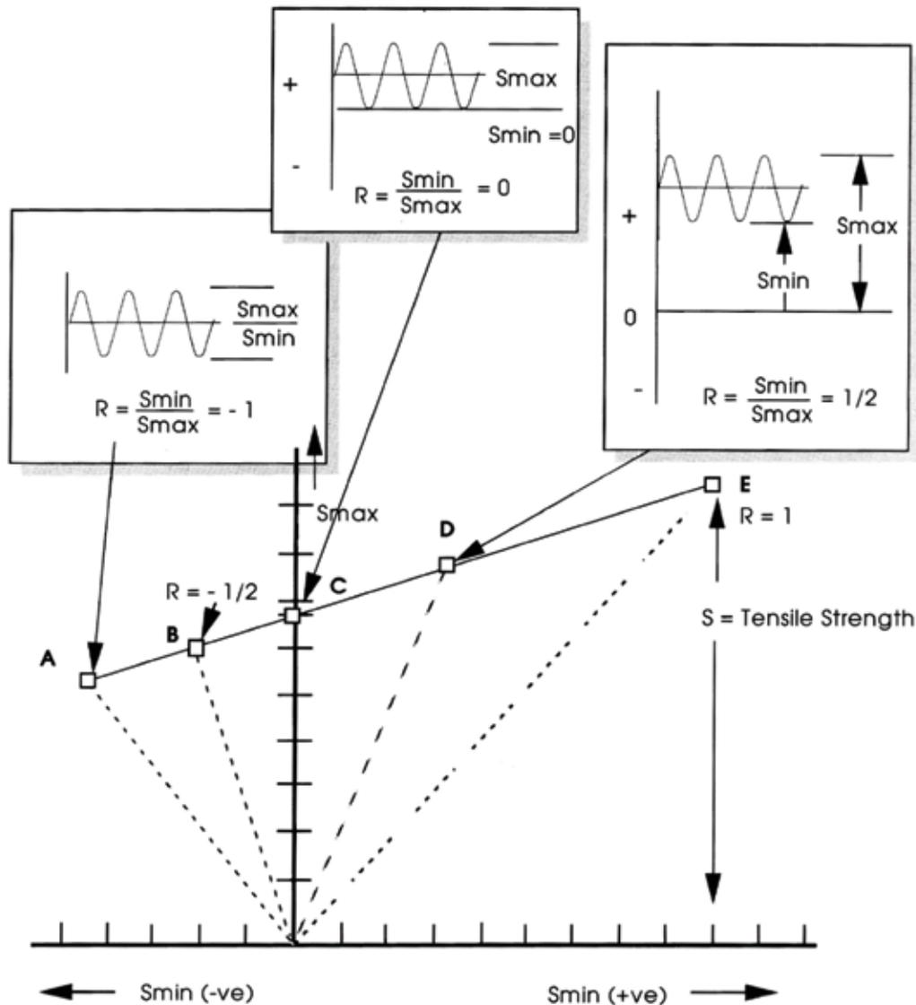
For example, after the application of a tensile load the specimen may simply return to zero stress before re-application of the tensile load. Alternatively, an applied static tensile load may be present and an alternating cyclic load may be superimposed. To differentiate between such loading conditions a convenient means to define the loading conditions is achieved by the use of the stress ratio,  $R$  which is defined as:
