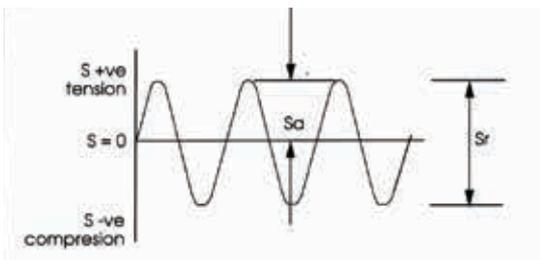
Fig 2 Diagram showing the sinusoidal type of pulsating load generally applied in laboratory type work (carried out to determine fatigue data).
