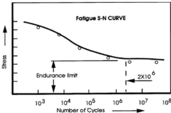
Fig. 3 Diagram showing the form in which data is presented, relating number of cycles to failure for a particular stress.
